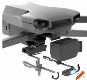
Figure 3. a. General concept of the accessory adapted to the drone, Modular transport structure (box/hook/clip), Remote release mechanism
