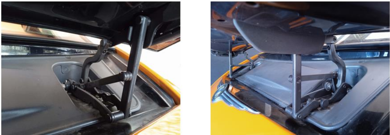
Figure 2. a. at the front it can be seen the crank-rod mechanism b. General view of the support mechanism
